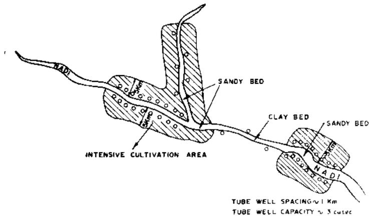
A schematic diagram for intensive cultivation by tubewell irrigation
