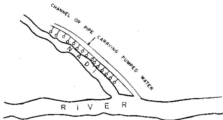
Augmenting river discharge (canal supply) with water pumped from Nadi bed during dry season
