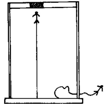
**Remarks :** It is desired that the magnet concealed in the wooden frame be of high strength (Alnico or ceramic magnet) since the force with which the pin is pulled up should be more than the weight of the pin itself.
