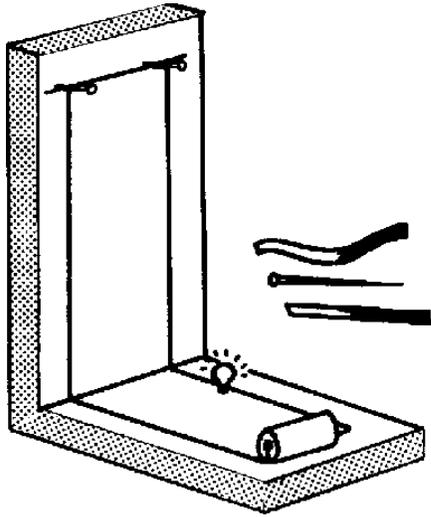
Equipment indicating electrical conduction through materials like wood, plastic, iron wires, etc. The equipment has a torch battery attached to electrical circuit. The electrical circuit is incomplete having two ends A and B, when two terminals A & B are connected by materials like iron or aluminium the circuit becomes complete and the bulb on the line lights up. If the material is a bad conductor, the light does not light up
