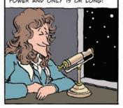
NEWTON'S SECOND, LARGER RE-FLECTOR, LIKE THE FIRST, HAD A POLISHED METAL MIRROR THAT ABSORBED SOME 80% OF THE INCIDENT LIGHT.
