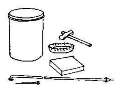
1.To make this pump you will need a film reel bottle, a bicycle spoke, a crown cap, a piece of rubber, a nail, an extra nipple nut, nail, hammer and some simple tools.
