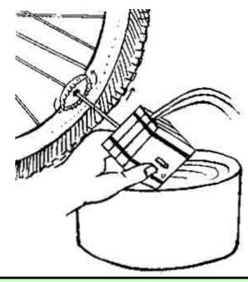
5. Dip the suction port in water and press the soda water cap against the rotating tire and enjoy the water gush out of the outlet.
