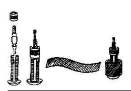
1. Take an old cycle tube valve body. Insert the valve stem and then screw the brass cap lightly. Insert a small matchstick piece in the bore of the valve stem. Take a 2 x 15-cm long piece of old tube rubber and wrap it tightly around the brass valve body.
