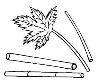
1.Can your convert a bamboo tube into a pump? Any hollow tube - a PVC or metal pipe, a short length of bamboo, or even a 30-cm long papaya stem can be made to pump up water. Take a short length of bamboo.
