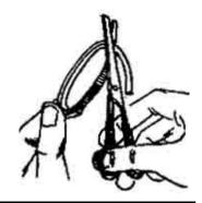
2. With a sharp scissors cut and remove the outer circle of the cap. The inner circle will make a superb piston. Rub it a little on sandpaper so that it is free inside the bottle — the cylinder.
