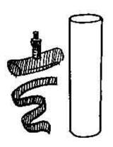
2. Take a 30-cm long PVC pipe with an outer diameter of 2.5-cm. Cut a strip from an old bicycle tube 2 x 20-cm long.
