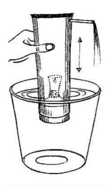
4. Hold the tube with your hand and move it up and down into a mug of water. After a couple of strokes water will start squirting out.
