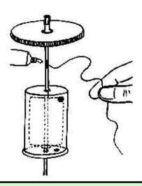
3. Tie 50-cm of thick but soft cotton thread to the spoke. Put a dab of rubber adhesive and tie a few knots so that the thread does not slip on the spoke. Now turn the flywheel a few times so that the thread loops around the spoke several times.
