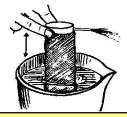
11. Now hold the lower bottle in water and press the top bottle B downwards. After a few initial strokes water will start gushing out of the delivery tube. Instead of pressing the top bottle up and down you can also squeeze it. Then the water will be squirted all around as in a sprinkler.
