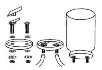
2. Make two holes in a jam jar lid. The holes should be the thickness of the cycle valve tube body. To prevent any leakage, cushion the lid with rubber washers on both sides, put a plastic milk bag strip on the left valve seat. Tighten both the valves to the lid with lock nuts. Attach two plastic hoses to the cycle valve bodies.
