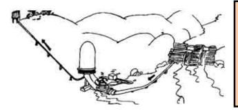
1. This pump, common in hilly areas, uses the water from a running stream and pumps it up. Theoretically it can pump water to almost 40 times the head between the pump and the stream. With this model you can raise water by almost one and a half meters.
