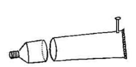
1. Old toothpaste tubes are not for throwing. Take a tube and cut it 2-cm from the mouth end. Clean it up. With a nail make a hole in the tube near the crimped base.
