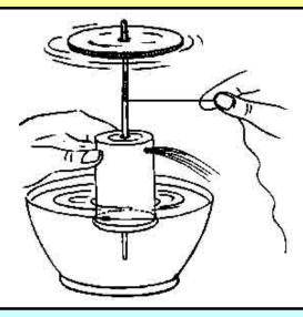
4. Keep the pump dipped in water in a vertical position and pull the thread. After a couple of pulls water will gush out of the pump and the flywheel will rewind the thread back on the spoke.
