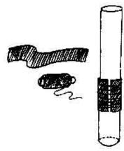
2 Take a 2-cm outer diameter and 30-cm long PVC pipe. Cut a 4 x 6-cm piece from an old cycle tube. Wrap just one layer of this tube on the PVC pipe and tie it with thread to secure it in place.
