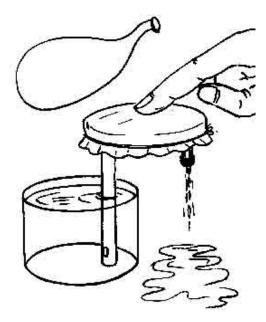
3. Now cover the lid with a torn balloon. Stretch the membrane and tie it tightly around the lid with a string. Tight fit a small plastic pipe - outer body of an old sketch pen to the left-hand valve. Make a hole in this pipe and immerse it in a vessel of water. Hold the rim of the lid with one hand and keep pressing and releasing the membrane with a finger. Soon water will be dripping out form the right hand valve.
