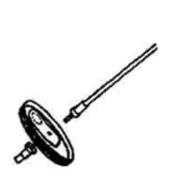
4. Cut a 12-cm long piece from a bicycle spoke. Fix the piston on the spoke thread with the help of two bicycle nipple-nuts.
