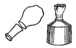
2. Cut a balloon about 2.5-cm from the mouth end. Stretch the mouth of the cut balloon and slide it on the threaded end of the mouth of the tube. This makes a very efficient valve.
