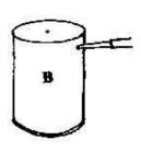
8. Take another film-reel bottle B and make a small hole on its cylindrical surface.
