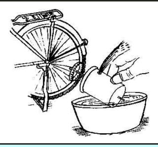
5. Keep the pump in an inclined position in a bowl of water, such that its inlet and outlet ports are diametrically opposite. Ask someone to put the cycle on the stand and crank the pedal. Press the crown cap of the pump to the rotating rubber tire. The rotor inside the pump will rotate very fast and water will gush forth with great force.
