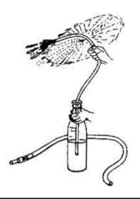
5. Water will keep sprinkling out as long as you continue spinning the tube. This way you can drain out the whole bottle. The centrifugal force of rotation is enough to suck and lift water from a height of almost a meter. You can make a simple foot valve using a cycle steel ball and a pen body as a seat.
