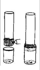
4. Take a 20-cm long PVC pipe with an outer diameter of 2.5-cm. Cut a 2 x 20-cm long strip from an old bicycle tube. Wrap the rubber tightly on one end of the pipe and secure it in place with rubber adhesive. This end of the pipe should be just fat enough to fit into the mouth of a film reel bottle. Insert the pipe in a film reel bottle, which has a flap valve in its base.
