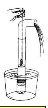
3. Hold the pump in water and reciprocate the cycle spoke. On each upstroke the suction valve opens sucking the water in the tube. The delivery valve remains closed. On each down stroke the suction valve remains closed and the delivery valve opens allowing water to rise in the PVC pipe and gush out of the bend with a great force.
