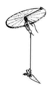
2. Hold the pen body in your hand and begin making circular motions - the potato must swing in a circle. As you increase the speed of rotation the carrot will rise. There is a force associated with the rotation of the potato. This force pulls away the center of the circle and is called Centrifugal force.
