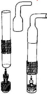
3. Insert the Delivery valve in the bore of the piston. The thickness of the wrapped rubber around the brass body should be such that it should be a tight fit in the bore. Also attach a bead to the top of the piston. It is through this bend that water will come out of the pump.
