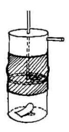
7. Make a 3-mm hole in the center of the bottle base so that the cycle spoke can move freely in it. Make another hole on the curved surface near the base and fix an old refill or *Frooti* straw in it. This is the delivery pipe.
