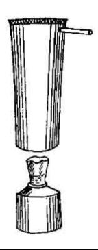
3. Insert this valve end in the big toothpaste tube as shown. Also insert a plastic straw (a *Frooti* straw or an old refill) in the hole near the crimped end. The cut balloon allows flow of water in one direction. Water can enter the tube from below but cannot come out from that end. The cut balloon is a very efficient valve.
