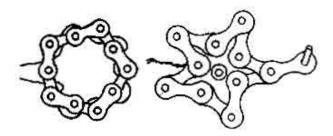
2. Weave a mild steel binding wire through the chain links and kink its two ends to make a five-pronged rotor. Rivet a link to any prong as a handle of the rotor
