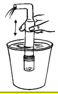
5. Attach a right angle bend to the top of the pipe.
