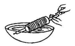
5. The pump is now ready for operation. Place it in an inclined position in a bowl full of water. The pump will turn about the left pivot nail - which will rest at the bottom of the bowl.
