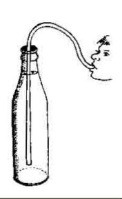
3. This simple sprinkler works on the same principle. Take a onemeter long flexible plastic tube - the one used as a petrol pipe or a mason's level tube. Keep one end of the tube immersed in a bottle of water and suck from the other end.
