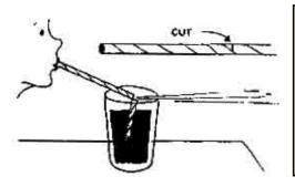
1.Make a slit in a plastic straw about one-third from one end. Bend the straw at the slit and place the short section in a glass of colored water. Make sure the slit is no more than 5-mm above the surface of the water. Blow hard through the straw. You will see that water enters the straw from the glass and comes out through the slit like a spray.
