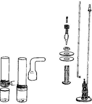
2. For the piston cut two circular pieces of cycle tube rubber so that they move snugly inside the PVC pipe bore. Make holes in the center of these washers and after inserting them in the valve body, tighten them with a lock nut, insert a little matchstick in the valve stem and assemble it in the valve body with the brass cap. Tightly tie a cycle spoke to the valve body with thread. The spoke becomes the connecting rod. Make a
