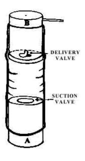
10. Cut a 15-cm long piece from an old cycle tube. Stretch and slide the tube over both the bottles as shown. The bottles will be separated by 7-cm of cycle tube. The rubber tube acts like a pair of bellows.
