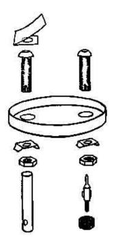
1.Make two 1-cm diameter holes in the lid of a jam jar. Slide a cycle brass valve tube body in each hole and fix them with a lock nut. Before fixing the left valve, wedge a plastic milk bag strip between the valve and the lid. This plastic flap acts like a suction valve. Tightly affix both valves to the lid. Insert the valve stem in the right hand valve and tighten the knurled cap screw on it.
